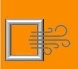
Divisible module for blowing pre-assembled cables and FTTH outlets into the microducts assisted by compressed air. This blowing unit is also suitable for blowing cables in two directions or from duct to duct, without splicing, smoothly and quickly.
