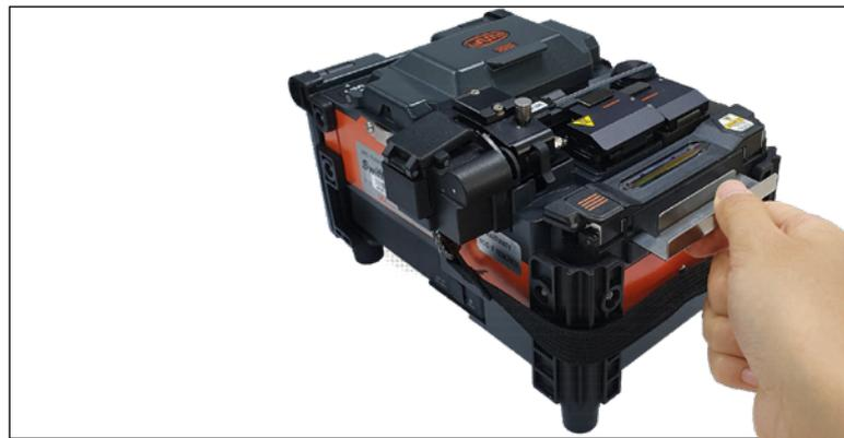
Install the cooling tray on the rear side of heater as above.
