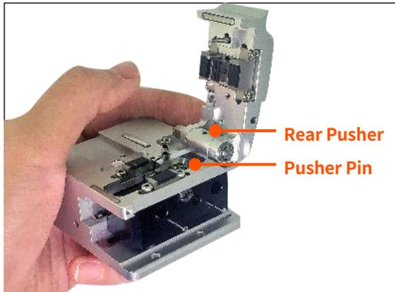
**1** In order to replace blade, disassemble chip collector assembly and rear pusher. Open the cover as shown picture and press the pusher pin to move slider to forward.
