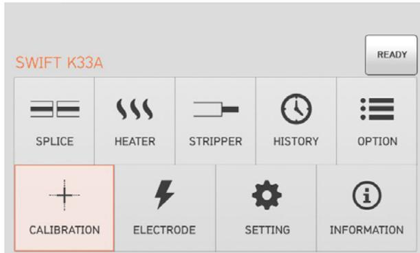
In normal operation mode, to call the calibration menu, press **MENU**. Then you can see the calibration menu as above. There're already various functions to arc test, diagnostic test and motor drive test.
