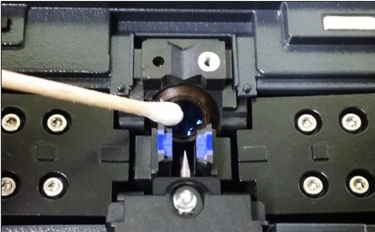
Contamination on object lens' surface disturbs distinction of optical fiber core's location and consequently incurs high splice loss. Thus, 2 object lenses should be kept clean at all times. If dust accumulates and is left for long, it may be difficult to remove. Therefore, clean the lens frequently as follows.
