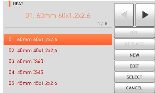
Choose the right mode for each sleeve tube type and SOC. Otherwise sleeve tubes do NOT shrink properly.
