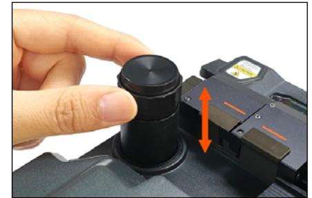
The alcohol dispenser in the Swift K33A has a limited capacity; the alcohol pump can be removed and refilled with cleaning fluid.
