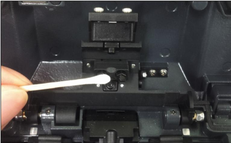
Contaminations remaining on Pusher Block incur poor splice quality with influence on pusher block location. Thus, it is important to frequently inspect and regularly clean it.
