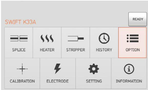
In normal operation mode, to call the option menu, press **MENU**. Then you can see the option menu as above. There're already various functions and whatever the user can select for proper operation.
