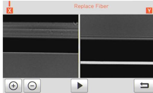
It is displayed when the fiber is not placed in the middle of the electrodes and V-groove or the objective lenses or reflection mirror is contaminated.
