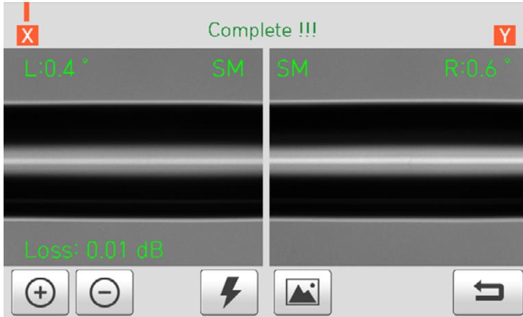
The condition of the fiber can be observed via the image processing system in the Swift K33A. However, the visual inspection is necessary to ensure better splice result. The splicing process starts as soon as the windshields cover is closed in Auto mode.
