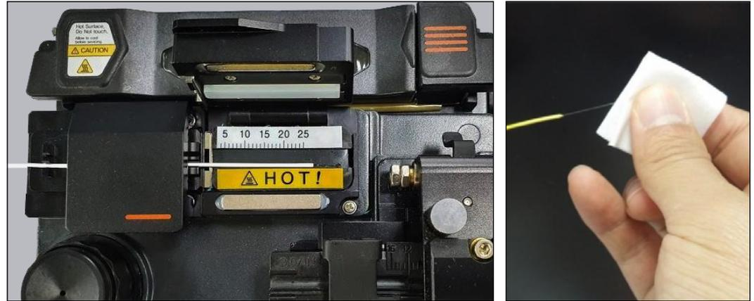
Do stripping procedure on about 26mm from the end of optical fiber by using Auto Thermal Stripper. And wipe the optical fiber clean with soft cloth or cotton moistened with alcohol.
