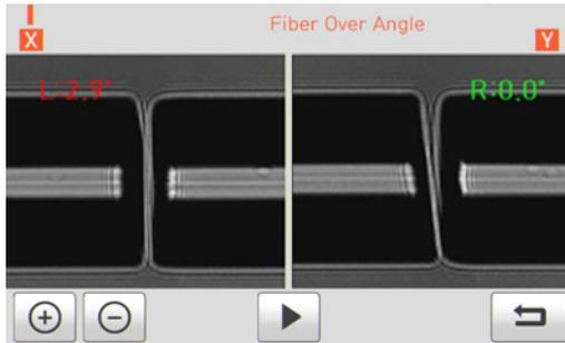
It is displayed when the measured cleaving angle of the fiber is greater than the limit.
