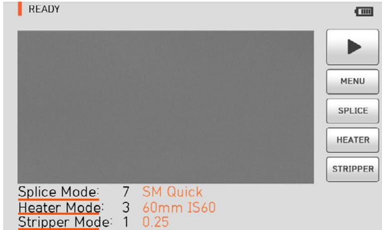
Press and hold for about 1.0 second without opening the windshield cover. The initial screen is displayed as above after resetting all their initial functions. It is important to choose a right splice and heat mode to ensure an accurate splicing result. The current splice, heater and stripper mode are displayed at the bottom of the initial page.
