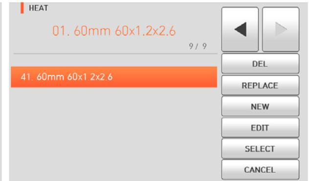
**3** The selected heater mode is added the last blank mode.
