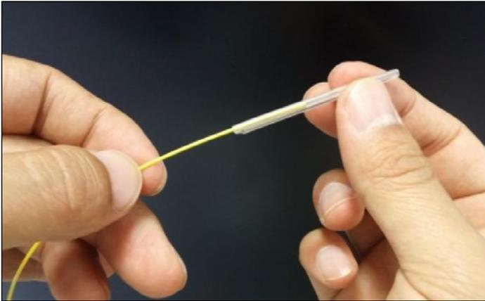
Insert the fiber into the sleeve.
