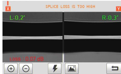
It is an error message generated when estimated loss value is higher than the preset loss factor limit.
