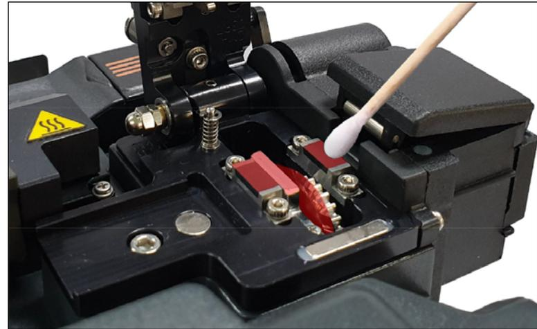
The performance of the fiber cleaver can be deteriorated if the blade or clamp pads of the cleaver are contaminated. In addition, the contamination of the fiber surface or tip can cause higher splice loss. For this reason, it is important to clean both the blade and clamp pads of the cleaver with a cotton swab soaked in alcohol.
