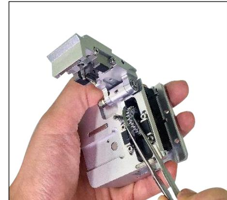
**3** Remove old blade with blade gear from body and replace new blade with blade gear. In here reassembling should be done in a reverse order of disassembling. At this time, especially be careful not to damage the blade. Check the blade operating condition with cleaver cover.
