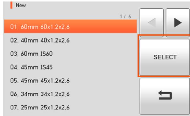
**2** Select the heater mode, click **SELECT**. The selected splice mode is added the last blank mode.
