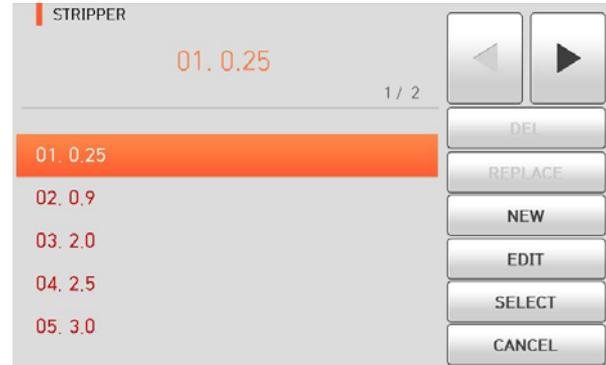
In normal operation mode, to call the Stripper mode, press **MENU**. There're already various Stripper mode and the user can select for proper operation. Also the heat mode will be stored up to 100.
