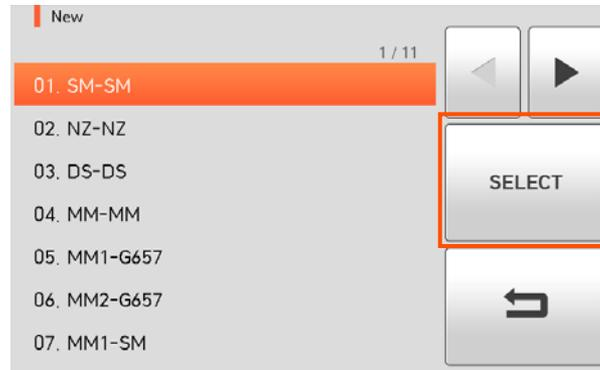
**2** Select the splice mode, click **SELECT**. The selected splice mode is added the last blank mode.
