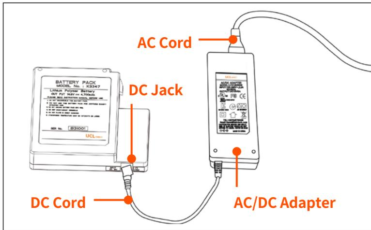
Make sure the voltage and frequency and connect the DC cord of the AC/DC adapter to the DC jack of the battery. The LED turns to green when the charging is completed. The battery includes the protection circuit that prevents full discharge and full charge. The supply of power stops once the protection circuit is activated. In order to deactivate the protection circuit and resume feeding power, wait about 10 seconds and connect again the DC cord to the DC jack.
