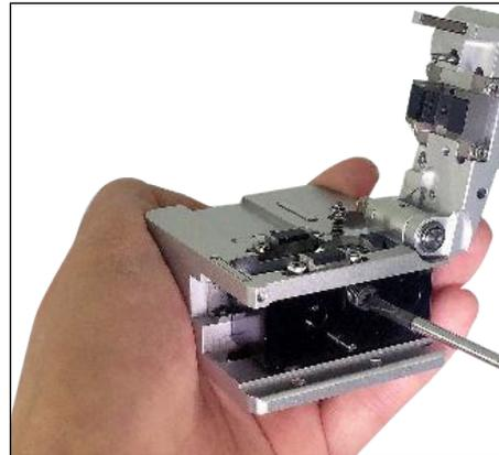
**2** Remove blade pin completely using (-) driver.
