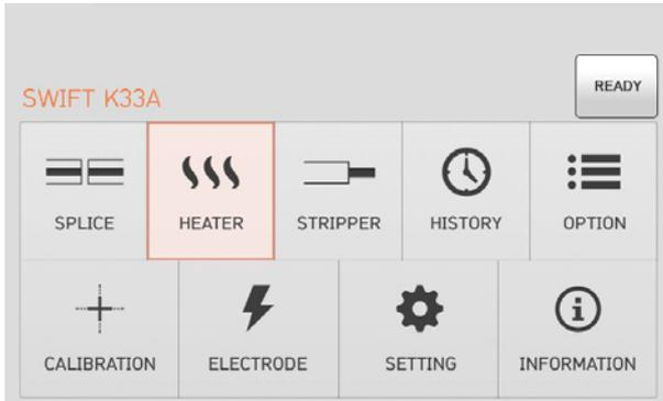
In normal operation mode, to call the heater menu, press **MENU**. Then you can see the heater menu as above.
