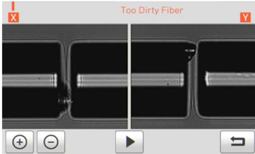
It is displayed when the fiber prepared for splice is contaminated more than normal status.
