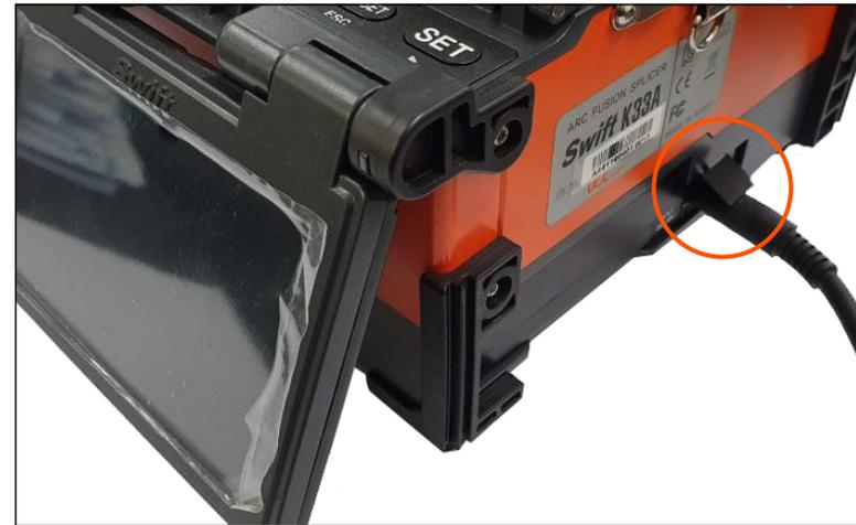
Swift K33A can be charged during operation because the floating charging method is applied. The battery can be also charged with 12V Cigar jack charger.
