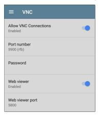
Allow VNC Connections: Tap the toggle button to enable or disable remote connections from VNC clients.
