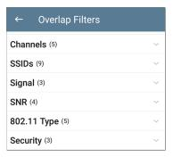
The number in parentheses shows how many active network characteristics are detected for each category. (The example shows (5) active Channels, (9) SSIDs, and so on.)
