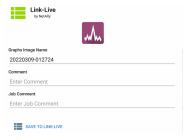
The Link-Live sharing screen opens. The system creates a file name automatically using the date. You can also enter optional Comments and Job Comments to attach to the results file. The results are displayed as images on Link-Live.com.
