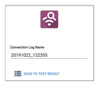
Tap the field to enter your desired log name, and tap **SAVE TO TEST RESULT** to upload.
