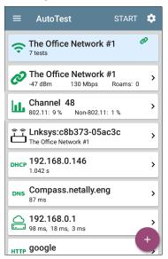
Like the main AutoTest screen, Wi-Fi Profile tests are summarized on cards. Tap a card to view individual test screens.
