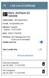
The buffered files displayed automatically upload to Link-Live.com once your AirCheck G3 connects to an active network.
