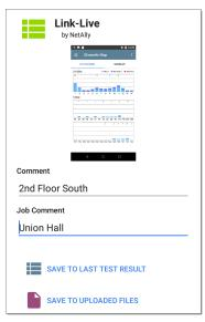
The **SAVE TO LAST TEST RESULT** option attaches the image to your most recently run AutoTest or iPerf results on Link-Live.com.
