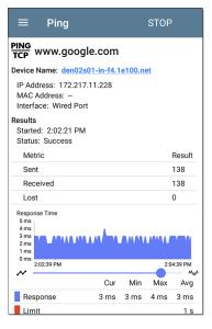
**Device Name**: Hostname or address of the target device
