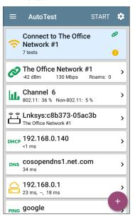
This Profile connects to SSID "The Office Network #1." The Profile is displaying one Warning condition from a timeout of the second Gateway ping.
