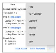
Tap blue links or the blue action overflow icon at the bottom of the test results screens to run the DNS Test Again, open another app populated with the name and IP address of DNS 1, or Browse to the Primary DNS server in your web browser.
