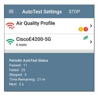
The Periodic AutoTest Status is summarized at the bottom of the AutoTest screens. Passes and failures are reported for each run of the entire Profile Group, rather than individual Profiles. Periodic AutoTests are skipped if the previous interval's test is still running when the next time interval occurs, such that the next run could not start.
