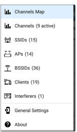
The Wi-Fi app's navigation drawer displays a real-time count (in parentheses) of each wireless component AirCheck G3 has detected. Tap an option to open the corresponding screen.
