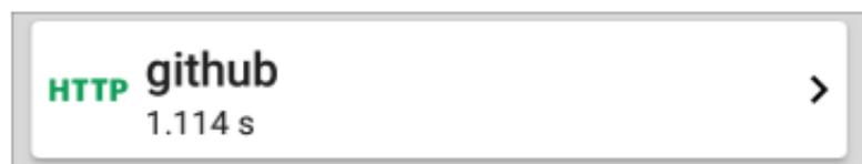
The HTTP card shows the test name entered in the test settings and response time from the target.
