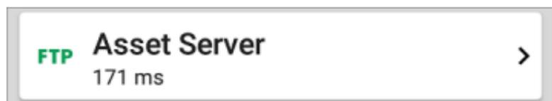
The FTP card shows the test name entered in the test settings and response time from the target.
