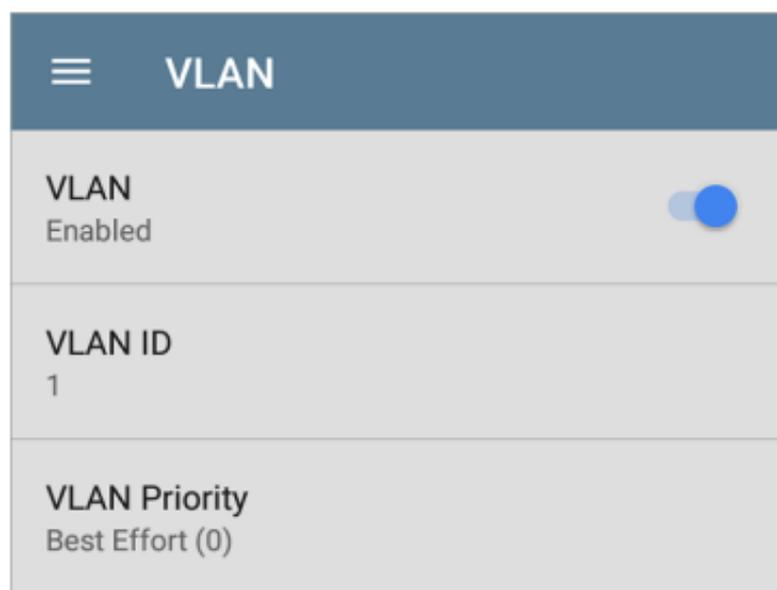
Tap to open the VLAN settings screen. Slide the toggle to the right to enable VLAN testing. Enabling this setting also enables a [VLAN test card](#) on the Wired AutoTest results screen. Once enabled, **VLAN ID** and **VLAN Priority** fields appear. Tap these fields to open a pop-up number pad and enter the correct ID and priority. Tap **OK** to save them.
