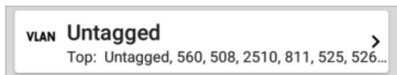
Untagged indicates that no VLAN tag is present in either received or transmitted frames, also referred to as the Native VLAN.
