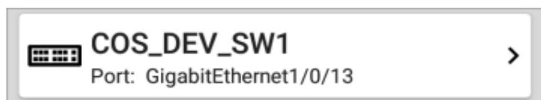
The Switch test card displays the Nearest Switch and the port name. The Switch icon remains black if the test is successful.
