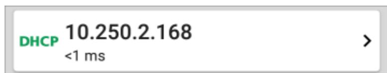
The DHCP Test card displays the DHCP server's IP address and the total time for the discover, offer, request, and acknowledgment to complete.
