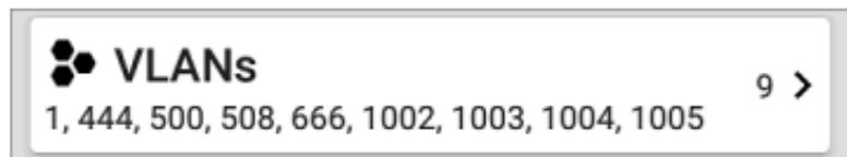
This card does not appear if no VLANs are detected or configured. Tap the card to open the VLANs screen.
