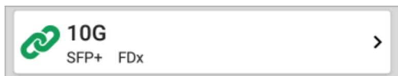
For a Fiber connection, the Link test card shows the connection speed and duplex.
