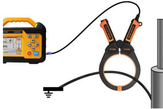
Figure 26 Running cable clamp coupling Method 2 (Clamp cable ground wire)
