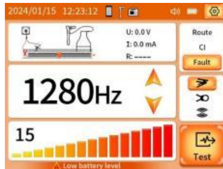
Figure 64 Transmitter fault finding interface
