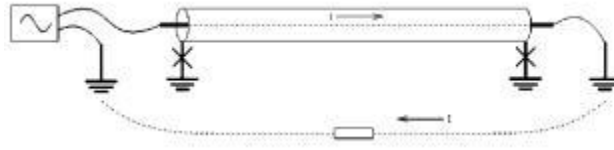
Figure 13 Schematic diagram of the signal flow direction of the core-ground method
