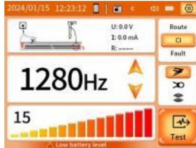
Figure 10 Output interface of cable identification mode direct connection method
