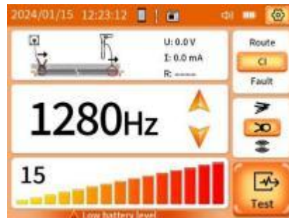
Figure 22 Cable identification mode clamp coupling output interface
